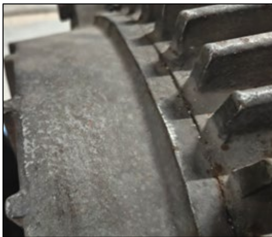
Figure 6: Surface cleaning with sandpaper
