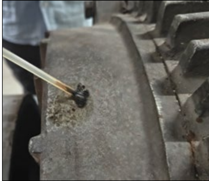
Figure 7: Activator applied on surface
