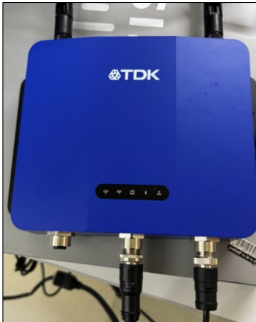
Figure 12: Gateway with power connected
