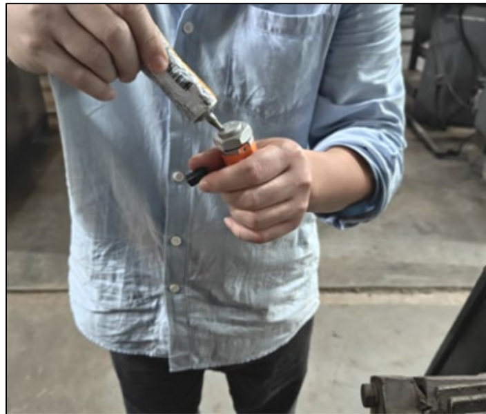
Figure 8: Adhesive applied on sensor base
