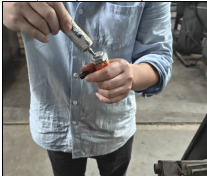
Figure 8: Adhesive applied on sensor base
