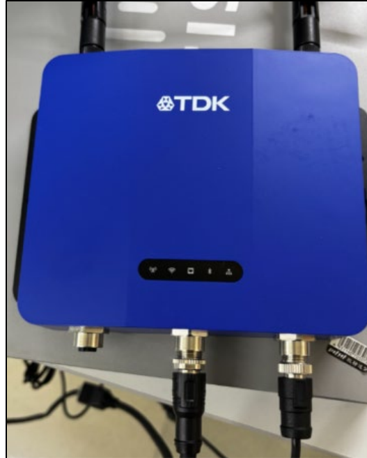
Figure 12: Gateway with power connected
